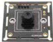
ELP-USB100W07M-MHV45 Small size 32x32/26x26mm, small M7 lens, well used for small space, door bell and button system,credit card machine, attendance machine....
