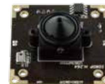
ELP-USB3MP01H-L37 3MP, WDR camera, H.264 Application: Traffic monitoring, Packing lot, Packing entrance, ATM machine, traffic toll gate ...
