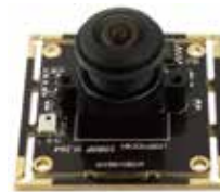
ELP-USBFHD04H-L180 2MP H.264 USB camera, wide angle With microphone, can record audio Well used for video conference, robotic vision system...
