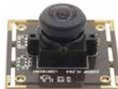
ELP-USBFHD06H-L180 2MP, Sony sensor, H.264, 0.01 LUX low illumination , wide angle Best choice for weak light condition, but no need LED.
