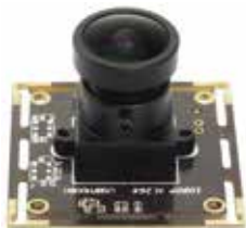
ELP-USBFHD06H-L 170 2MP, Sony sensor, H.264, 0.01 LUX low illumination , wide angle Best choice for weak light condition, but no need LED.
