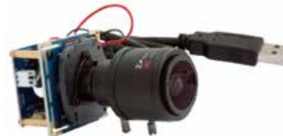
ELP-USBFHD01M-FV 2MP, 2.8-12mm varifocal lens, Mjpeg 30fps@ 1080P, 60fps@ 720P, 120fps @ 640x480 VGA
