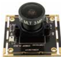
ELP-USBFHD04H-L170 2MP H.264 USB camera, wide angle With microphone, can record audio Well used for video conference, robotic vision system...
